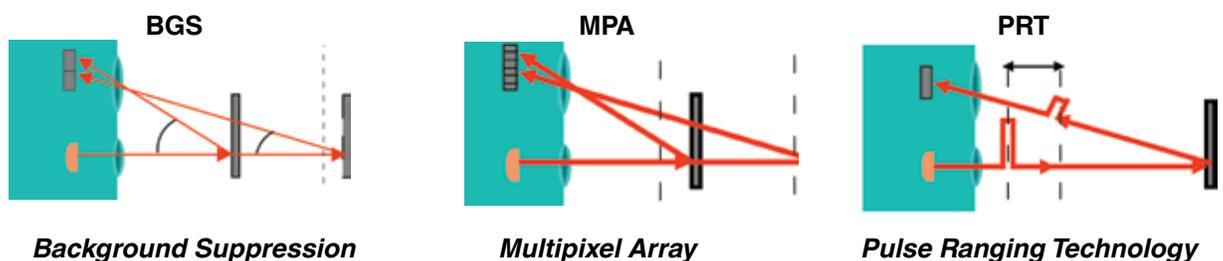
Figure 1. Three methods of distance-based photoelectric sensing
