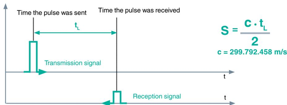
**Figure 2.** Principle of operation of a PRT distance measurement sensor. The sensor transmits a short intense burst of light that travels to an object and is reflected to its receiver. The time for the reflected light to return to the sensor's receiver ( $t_L$ ) determines its distance ( $s$ ), with the speed of light as constant  $c$ .
