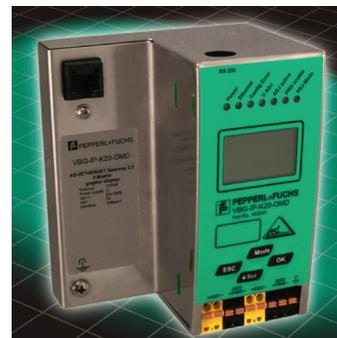
*An AS-Interface gateway enables upper-level networks such as Ethernet to benefit from the strengths of AS-Interface. As far as the upper-level network is concerned, the AS-Interface gateway is a large collection of I/O. Gateways are Masters for I/O nodes on AS-Interface, and slaves (or servers) on Ethernet.*
